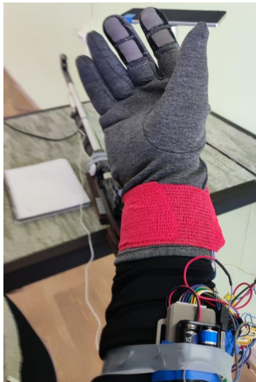
Figure 1. Smart glove connected to data acquisition unit
